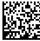
Figure 13. EAN/UPC encoding GTIN, and GS1 DataMatrix encoding both GTIN and secondary information (i.e., Production Date, Batch/Lot, Number, Serial Number)
