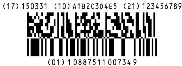
Figure 30. GTIN Encoded in GS1 DataBar (Limited), and Expiration Date, Batch/Lot & Serial Number Encoded on Composite Component
