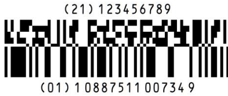
Figure 25. GTIN Encoded in a GS1 DataBar (Limited) & Serial Number Encoded in the Composite Component
