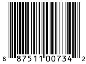
Figure 11. GTIN Encoded in an EAN/UPC, and GS1 DataBar encoding both GTIN and Expiration Date
