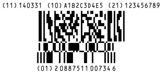
Figure 29. GTIN Encoded in GS1 DataBar (Stacked), and Production Date, Batch/Lot & Serial Number Encoded on Composite Component
